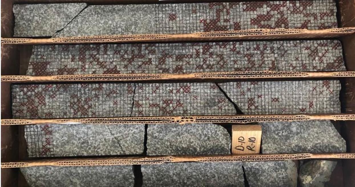
Figure 3: 1.5m sample interval, from 406m depth to 407.5m depth in drill hole 16TK0242, was broken down into a 1/4" grid and marked where sulphide minerals were visually observed
