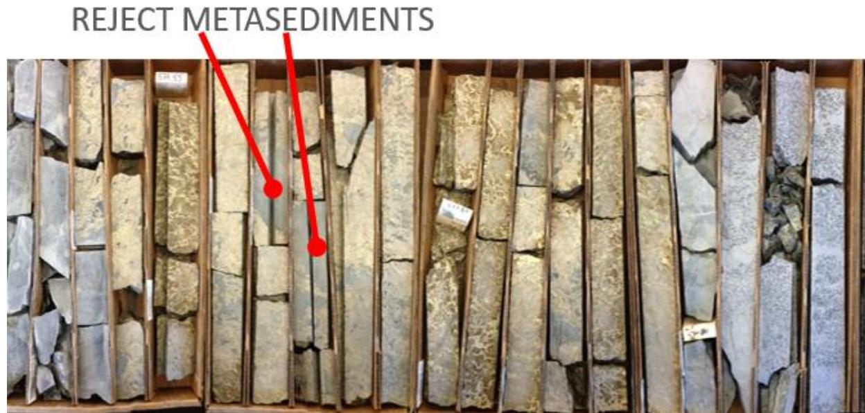
Figure 2: Image showing Metasediment and Mixed Massive Sulphide (MMS) units from drill hole 13TK0171, from 573.3m to 580.8 meters depth
