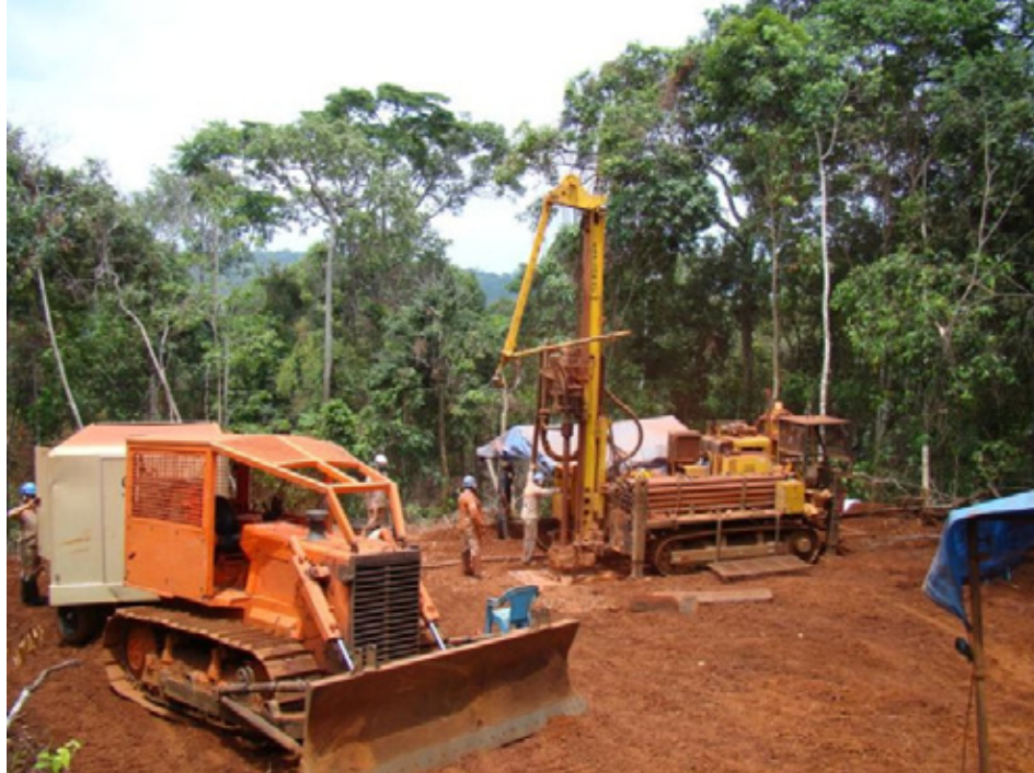
Figure 11_2 Trairão Iron Ore Project Drill Rig Explorac R50
